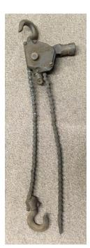
Tools serve as an extension or expansion of our physical capabilities. They reduce physical strain and allow us to do a job more efficiently. One of Margelony's block and tackle devices can lift up to two tons. This Coffin's Hoist Jack has two hooks. One is attached a sturdy place above a load. The other is attached to the load itself. A lever within the tool's housing is moved up or down to move the chain that lifts or lowers the load.
