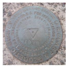
In July, surveyors funded by the WPA prepared a geodetic survey map of Connecticut. They placed several markers in the Rockville area showing elevations which were used for reference points on property deeds. This marker on the left can be found embedded in the walkway to the War Memorial Tower in Henry Park.
