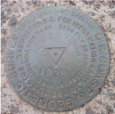
In July, surveyors funded by the WPA prepared a geodetic survey map of Connecticut. They placed several markers in the Rockville area showing elevations which were used for reference points on property deeds. This marker on the left can be found embedded in the walkway to the War Memorial Tower in Henry Park.
